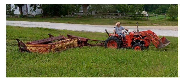
A "new" old piece of equipment at SHF. This Mower-conditioner not only cuts the hay, but then conditions the hay by crimping the hay via rollers that promote moisture evaporation and faster drying. It cuts down on the time needed for baling. With all the rain...we need faster drying!!!
